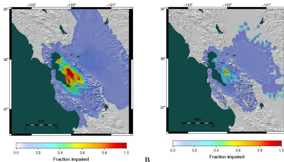
**Fig. 1 – Building impairment in M 7.0 Hayward Fault earthquake: (A) life safe ( $I_e = 1.0$ ) and (B) resilient ( $I_e = 1.5$ ) buildings**
