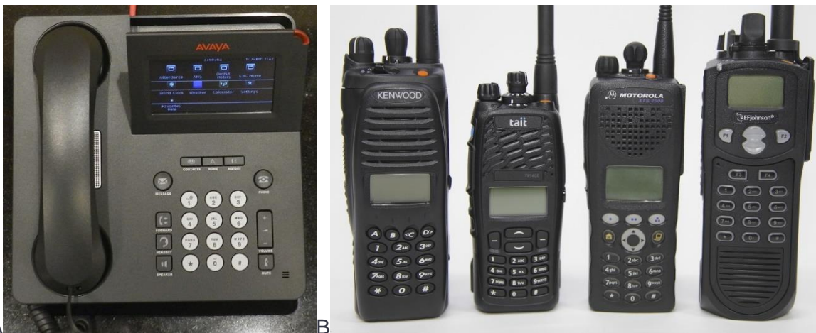
Figure 1. Audible warning for selected personnel can be delivered by (A) IP telephones or (B) two-way radios. (Images: A: Geek2003 Creative Commons Attribution-Share Alike 3.0 Unported, B: Evan Forester, public domain)
