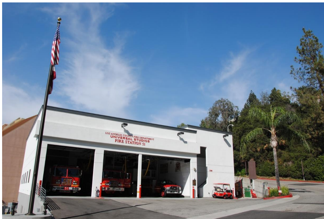
Figure 6. Earthquake early warning can automatically open fire station bay doors and sound an audible alarm through the fire station public address system, two-way radio system, or both (image: anonymous, CC-BY-SA 4.0)
