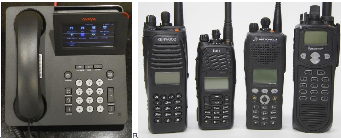
Figure 2. Audible warning for selected personnel can be delivered by (A) IP telephones or (B) two-way radios. (Images: A: Geek2003 Creative Commons Attribution-Share Alike 3.0 Unported, B: Evan Forester, public domain)
