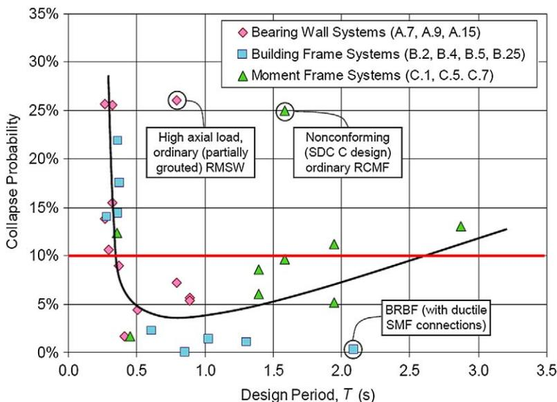
**Figure 1.** Collapse probability in  $MCE_R$  shaking in 179 buildings examined in *FEMA P-695* and *NIST GCR 10-917-8* ([NEHRP Consultants Joint Venture 2012](#)).
