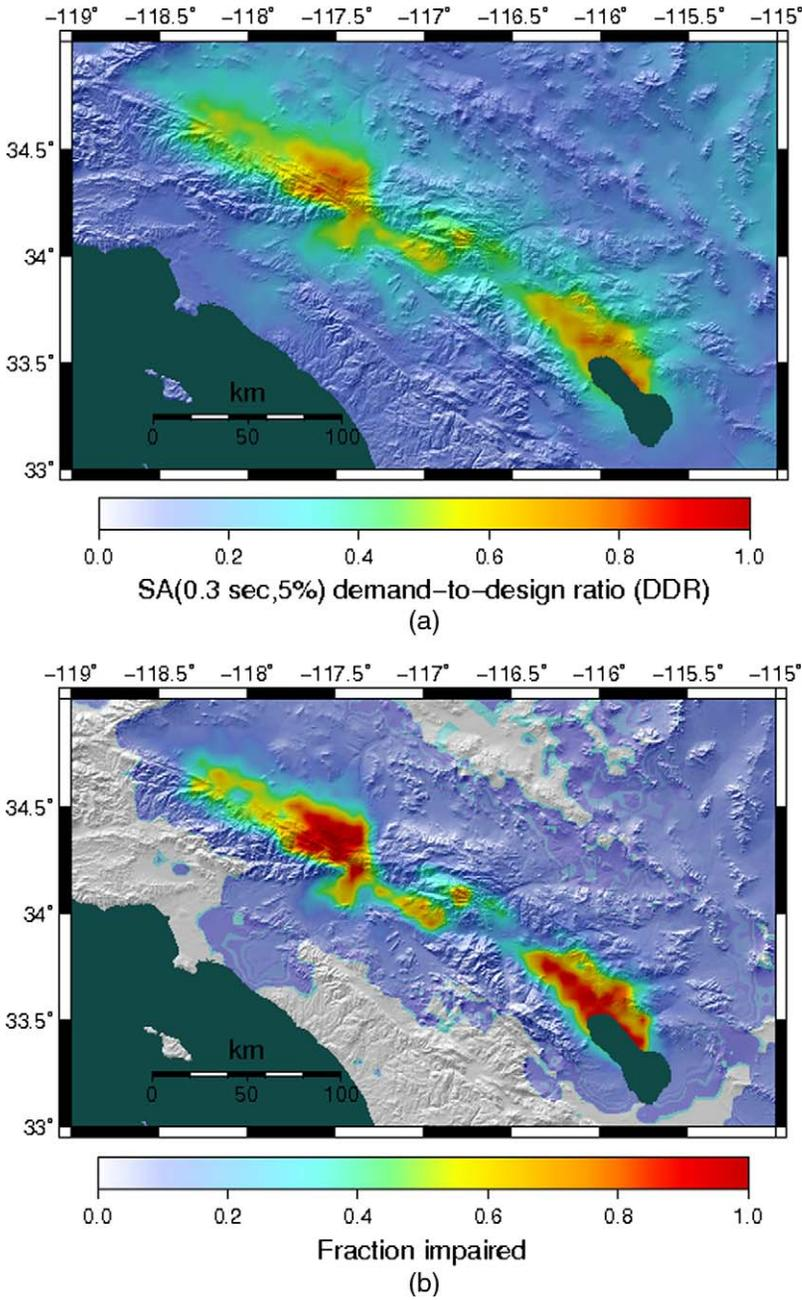
Figure 4. (a) Demand-to-design ratio *DDR* in the ShakeOut and (b) fraction impaired.
