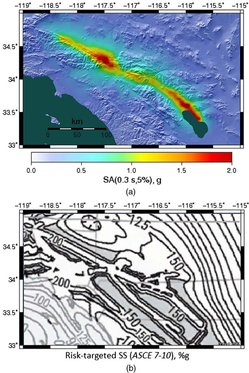
**Figure 3.** (a) ShakeOut  $S_a$  (0.3-s, 5%) compared with (b)  $S_S$  from ASCE 7-10. Shaking exceeds 0.5  $MCE_R$  shaking over roughly 10,000  $km^2$ .
