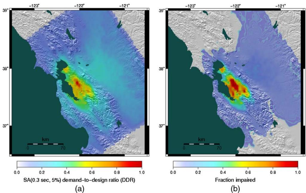
**Figure 5.** (a) Demand-to-design ratio for M 7.0 Hayward Fault scenario and (b) fraction of lowrise buildings impaired (collapsed, red- or yellow-tagged) under this scenario.
