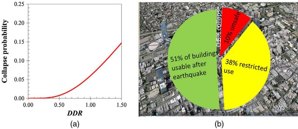
**Figure 2.** (a) Collapse probability as a function of demand-to-design ratio; (b) approximately half of the building stock is impaired at shaking of  $DDR = 0.5$  (i.e., one-half  $MCE_R$ ).
