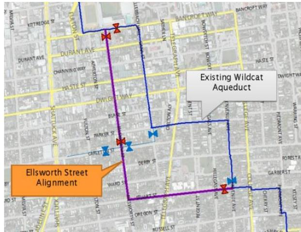
**Figure 6. Wildcat Transmission Pipeline.**
